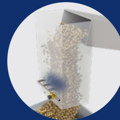
CONVENTIONAL EXTINGUISHING SYSTEM
